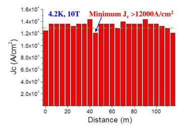
FIG. 2 The distribution of critical current density  $J_c$  throughout the 115 m long Sr122 wire.
