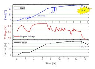
**Fig. 2** Test results in liquid He at 4.2 K. About 15 hour after the start of ramping the magnet reached 26.4 T (top blue line) at a power supply current of 242 A (bottom black line).
