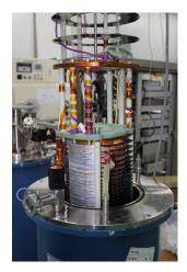
Fig. 1 Assembled magnet and liquid He Dewar.
