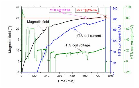
Fig.2. Test of the REBCO insert under 15 T background magnetic field at 4.2 K
