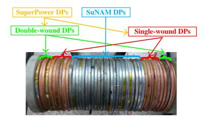
Fig.1. REBCO insert in assembly
