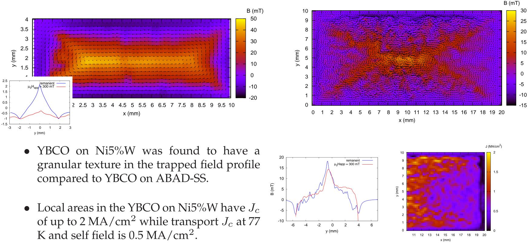
The critical current density is evaluated from the measured magnetic field profile by an algorithm that inverts the Biot-Savart Law:
