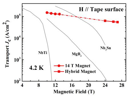
**Fig. 1.** Magnetic field dependence of transport  $J_c$  for the hot-pressed Ba-122 tape at 4.2 K. The transport  $J_c$  of other wires or tapes are also included for comparison.
