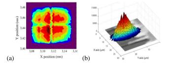
**Figure 1** SNSPD development at Glasgow (a) photoresponse map of 60  $\mu$ m x 60  $\mu$ m area four-pixel SNSPD array with peak detection efficiency >40%. (b) waveguide integrated SNSPD [3].
