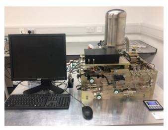
Figure 2 Miniaturized 4 K cooler for SNSPDs developed in partnership with STFC Rutherford Appleton Laboratory.
