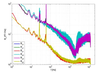
Figure 1: Unshielded noise of 2 high sensitive SQUID triples, acquired simultaneously NW of Delta, Utah, USA. Note the good correlation between the channels in parallel, obviously we mostly see external signal.
