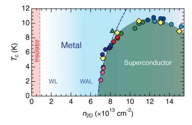
**Fig. 2**: Superconductivity phase diagram of  $MoS_2$  EDLT: With increasing carrier density, a crossover from weak localization (WL) to weak antilocalization (WAL) was observed in magnetoresistance at 2 K. The dashed line indicates fit to the equation of the critical phase transition.
