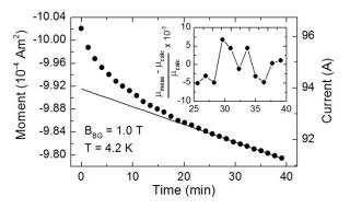
**Fig. 2.** The decaying magnetic moment of the sample coil as an induced current is attenuated across the joint. The current was generated by raising the field from 0.7 T to 1.0 T at 4.2 K. The solid line is an exponential fit to the settled trend with resistance  $R = 39.6 \pm 0.5 \times 10^{-15} \Omega$ . The inset shows the noise level on measurements in the fitted portion.
