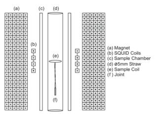
**Fig. 1.** A schematic illustration of the experimental setup, with the jointed sample coil loaded axially in the MPMS, centered on the SQUID pickup coils.
