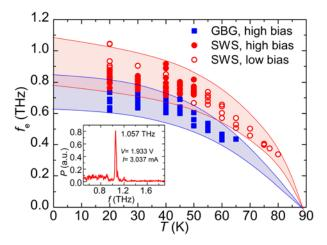
Fig. 2. Emission frequency vs. the bath temperature. The inset shows the spectrum of THz emission at  $T_b = 20$  K and I = 3.037 mA.
