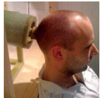
PhD student Fredrik Öisjöen prepares himself for proof-of-principle MEG recordings of his alpha-wave signals with one of our high-T c SQUID magnetometers housed in an epoxy reinforced glass-fiber cryostat from ILK Dresden. The measurements were performed inside a magnetically shielded room, courtesy Imego AB.
