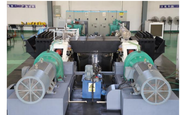
the world's first MW HTS induction heater
