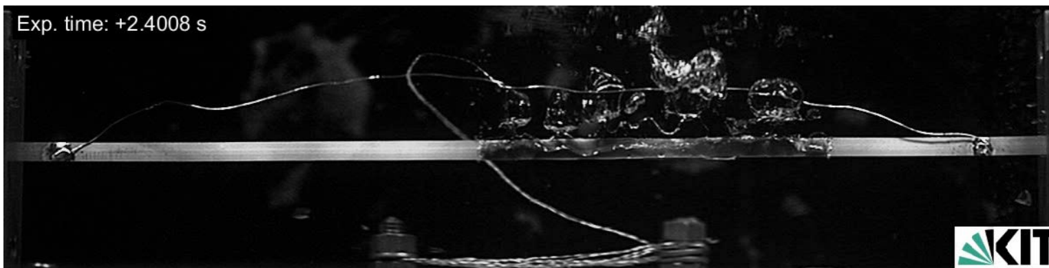
Superconductor 4mm, Superpower ReBCO-tape 40 \mu m Cu-stabilization
