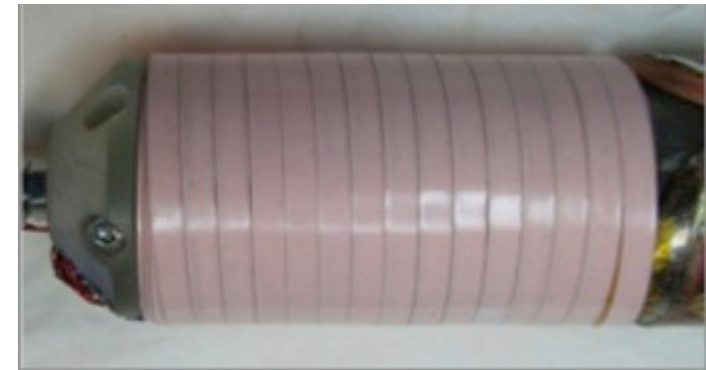
The 4.4 T REBCO insert that reached 35.4 T at NHMFL 2012
