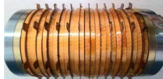
Assembly of the YBCO double pancake and installed in the LTS configuration
