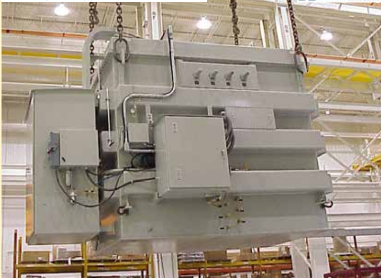
1MVA prototype transformer
