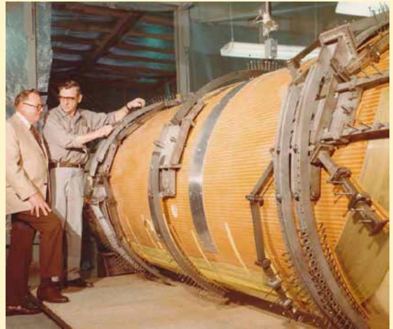
MT-5 Rome (1975) High Current DC Homopolar Generator using Carbon Fibre Brushes AD.Appleton IRD Ltd UK carbon fibre brushes in 1MW superconducting generator + motor for marine propulsion
