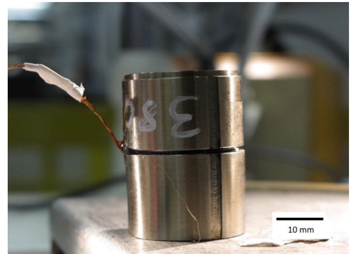
Stack of 2 x GdBCO samples that achieved 17.6 T at 26 K
