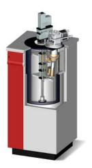
**Fig. 5.** The MPMS EverCool dewar and cabinet assembly. The 1<sup>st</sup> stage of the cryocooler is attached to the thermal shields in the dewar, while the second stage recondenses the helium gas that would otherwise be lost.
