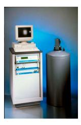
**Fig. 3.** An early PPMS system. This instrument is shown with the sample drive mechanism (on the top of the dewar and probe assembly) that provides the sample motion for the PPMS AC-DC Magnetization (ACMS) measurement option.
