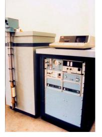
Fig. 2. The Mark I – the first Quantum Design MPMS. This 2-Tesla MPMS used an SHE Model 30 SQUID controller and the user interface was written in BASIC on a Hewlett-Packard HP-85 computer. The system was shipped to Prof. Robert Shelton at Iowa State University in July 1984.
