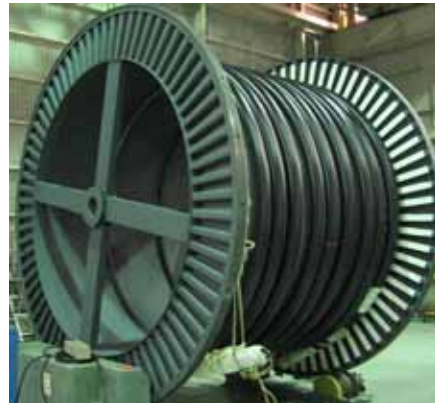
Figure 3. 30-meter HTS cable wound on a drum after manufacture.
