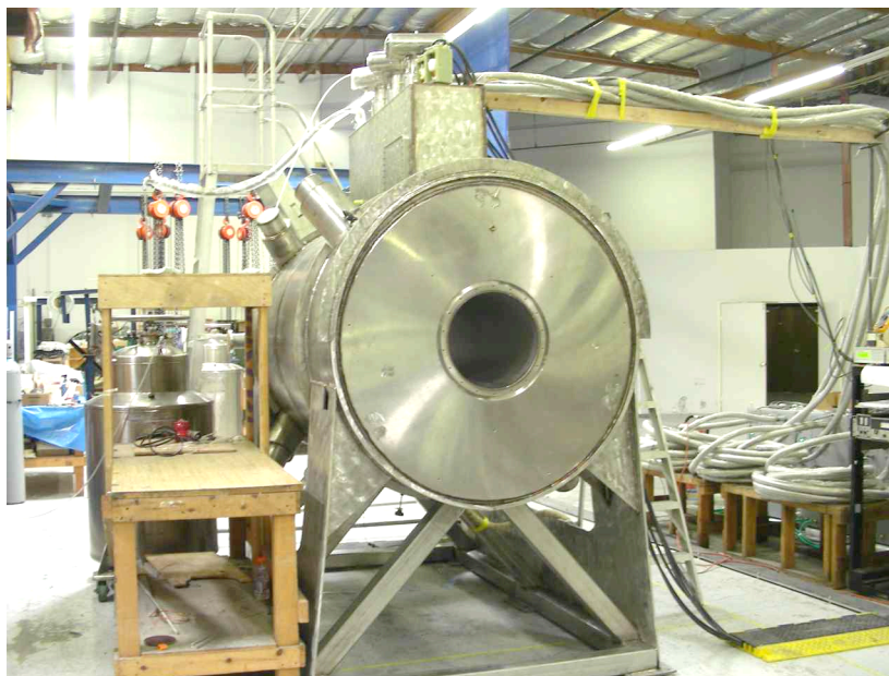
Figure 10. The finished first spectrometer solenoid during the magnet test (July 2008).
