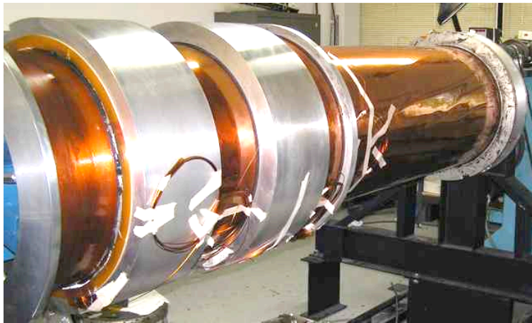
Figure 8. The winding of spectrometer magnet one (summer 2007).
