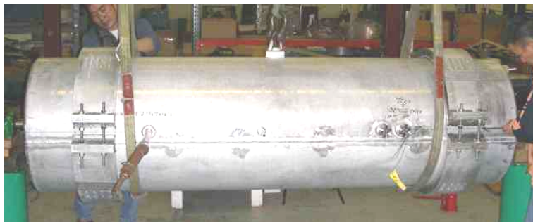
Figure 9. The completed magnet one cold mass assembly (fall 2007).
