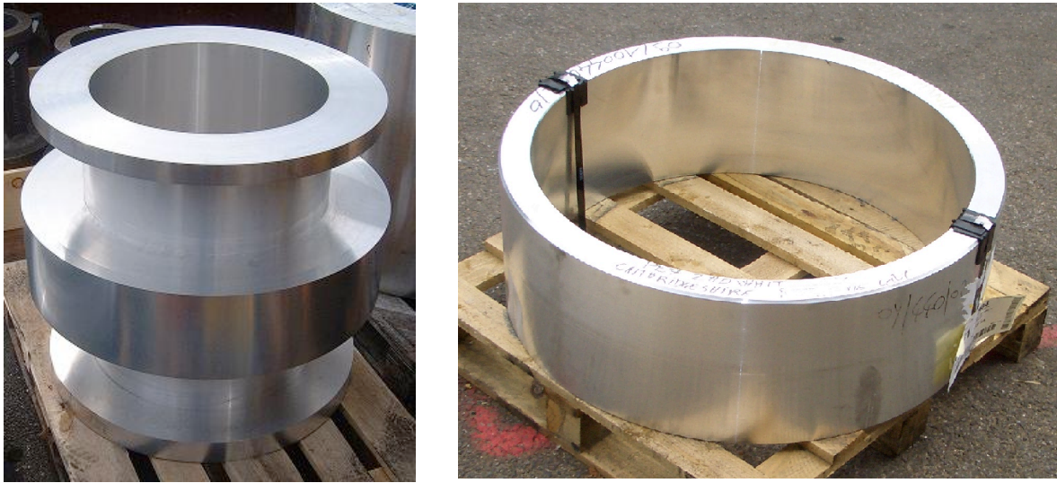
Figure 19. A rough machined focusing magnet mandrel (left) and a forged cover plate (right).
