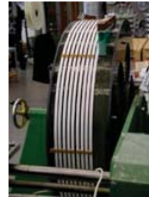
Testing superconducting high-current generator cable at Siemens
