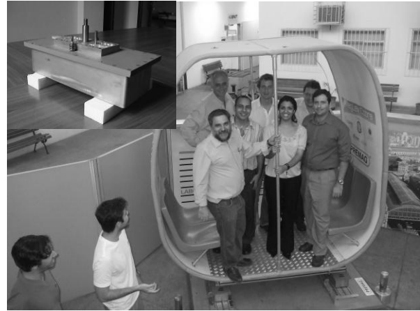
Fig. 8. Full-Scale Module of the Maglev-Cobra HTS-Superconducting Vehicle, U. Rio de Janeiro; Insert: MAGLEV HTS cryostat (ATZ).
