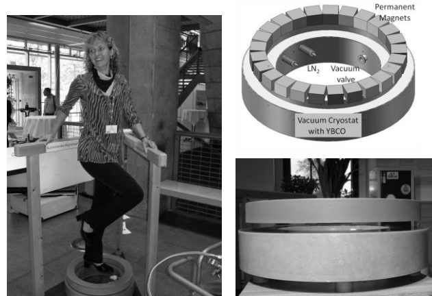
Fig. 11. HTS magnetic platform demonstrating levitation forces.
