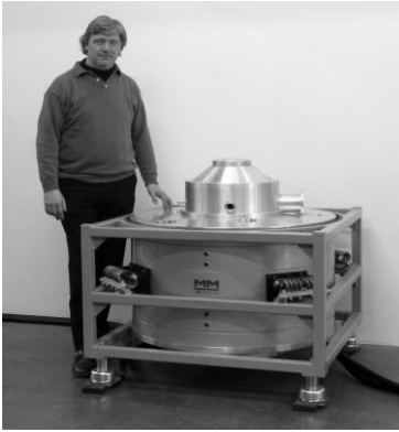
Fig. 4. ATZ/MM flywheel with HTS magnetic bearing.
