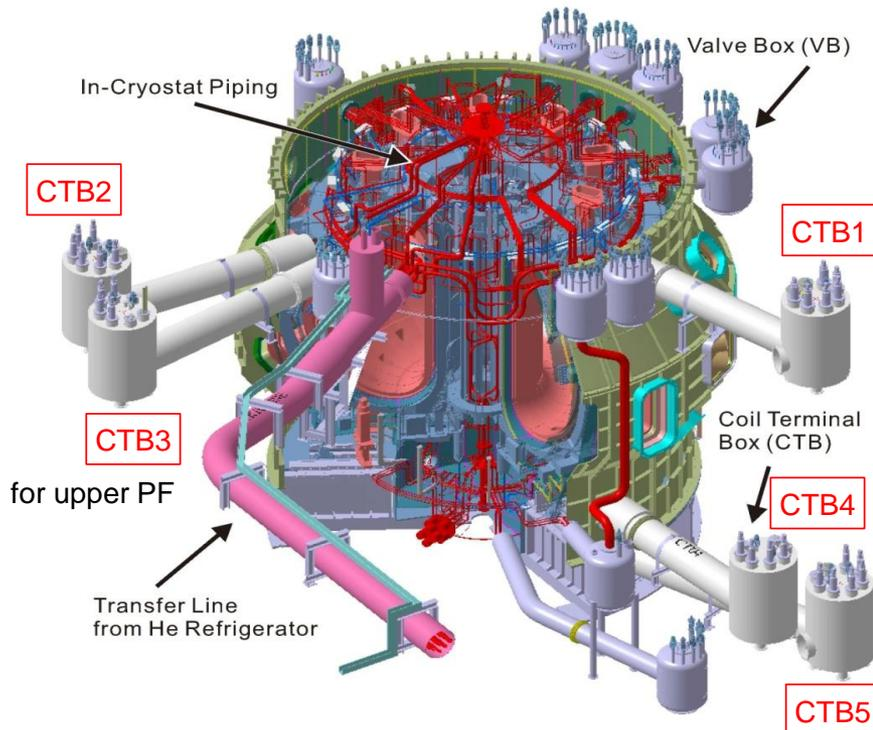
Cryogenic system for JT-60SA
