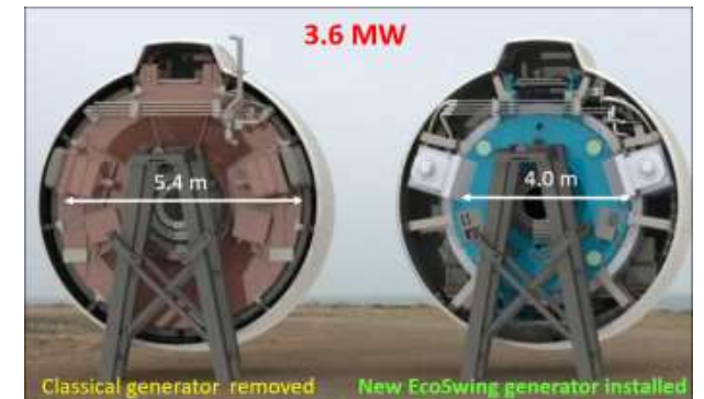
Old and new generator in same casing
