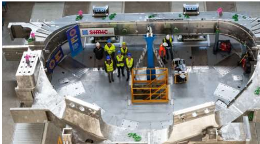
1 st TF coil in casing, closing welding
