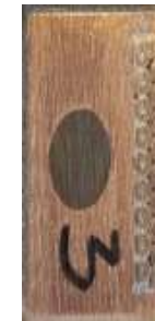
NbTi/Cu Rutherford cable in Copper bar, sf He in 6 mm hole for cryo-stability
