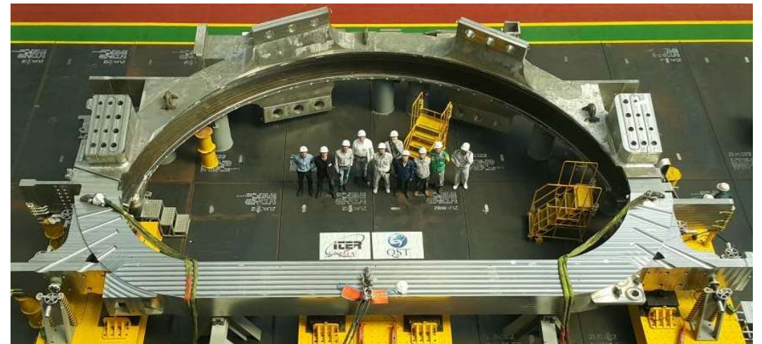
Coil casing completed, ready for the casing
