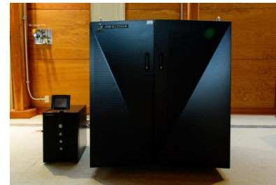
JNM-ECZ series NMR spectrometer
