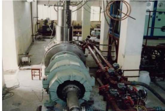
Fig. 2. Industrial prototype of 3 tons/h superconducting magnetic separator for kaoline clay purification.
