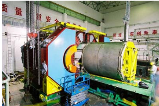
Fig.7. Superconducting Magnet for Beijing Spectrometer Detector
