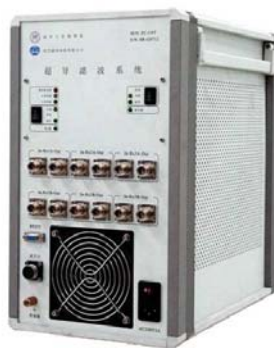
Fig.20. Superconducting Filter System for CDMA mobile telecommunications base station (Tsinghua Univ.)
