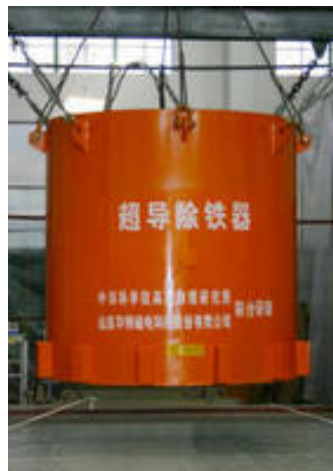
Fig.8. Magnet of the superconducting de-ironing separator.
