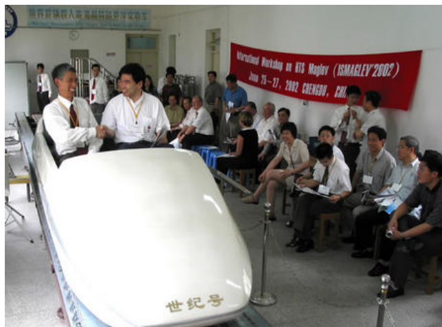
Fig.18. First man-carrying HTS magnetic levitation experimental vehicle.
