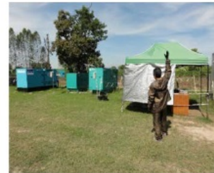
Signals for operating the generator
