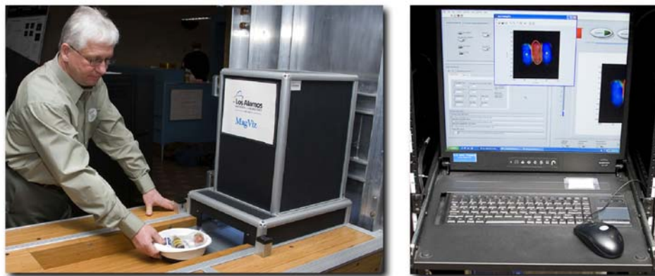
Fig. 5. Photos from actual operation: on the left samples being placed onto the conveyor. On the right a laptop screen shot showing detection of threat (red) material
