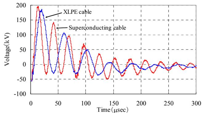
Fig. 5. Lightning surge voltage wave forms of HTS cable and conventional XLPE cable. Propagation speeds of HTS cable and conventional XLPE cable are 206 m/μs and 121 m/μs, respectively.
