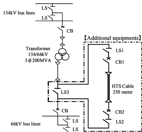
Fig. 2. Simplified power network diagram added the HTS cable and other equipment at the Asahi substation.
