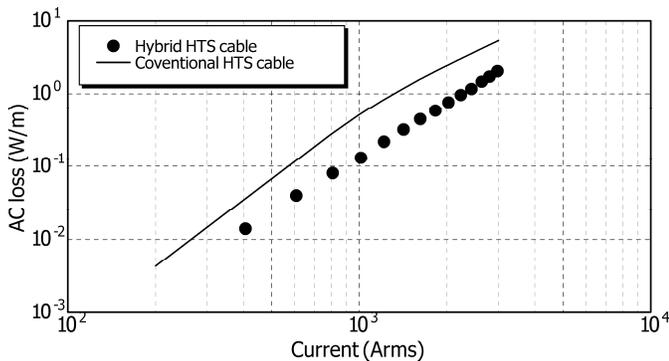
Fig. 7. AC loss test results for hybrid HTS cable core. AC loss of the hybrid core is much smaller than that of conventional cable core.
