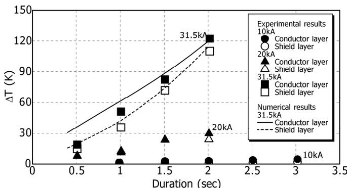
Fig. 8. Fault current test results of HTS cable core sample. Temperature rise ( $\Delta T$ ) was measured at the over-current flows of 10 kA, 20 kA and 31.5 kA under various time durations.
