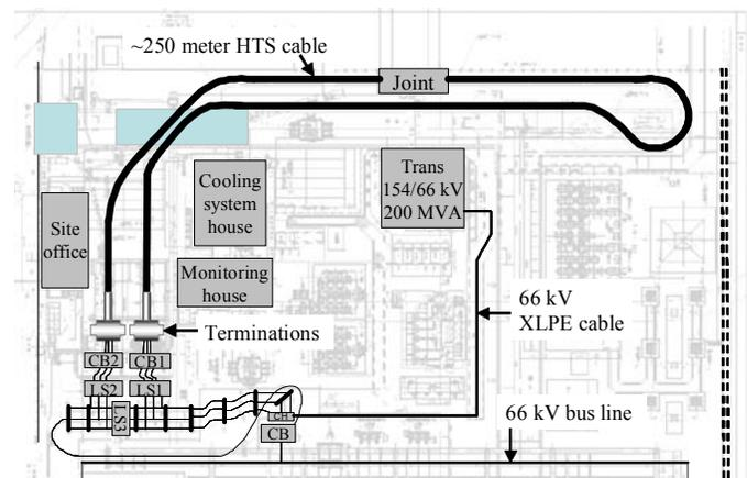
Fig. 3. Layout of the demonstration system in the Asahi substation.
