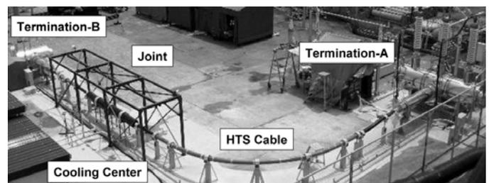
Fig. 9. Overview of the 30 meter HTS cable system.
