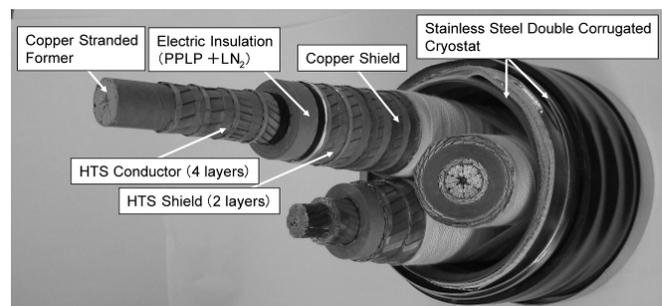
Fig. 6. HTS cable structure to be installed at the Asahi substation.
