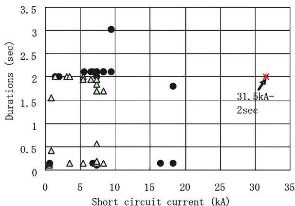
Fig. 4. Simulation results of fault current conditions. Circle and triangle plots correspond to non-rapid re-close case and rapid re-close case, respectively.
