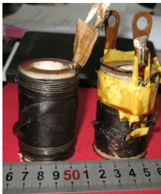
Fig. 8. Photo of the prototypes of coil 1 after winding and wiring.
