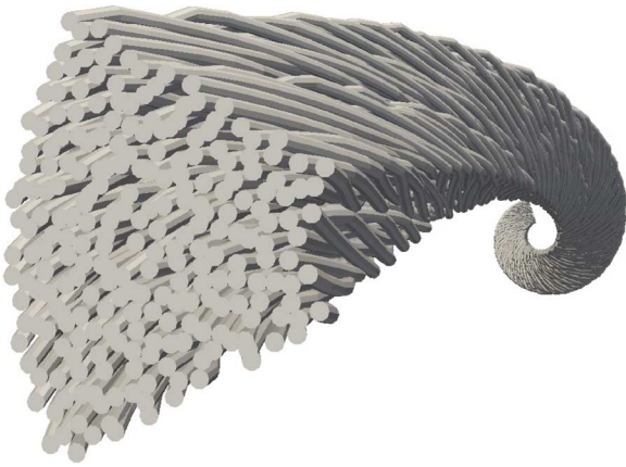
Fig. 6. Illustration of the coordinates of the 240 strands in the CICC used for the simulation of PF conductor.
