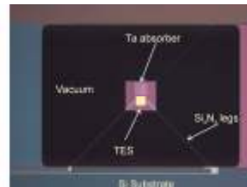
Fig. 4 TES #2 fabricated on 0.5 \mu\text{m} thick 160 \times 160 \mu\text{m}^2 SiN island supported by 1 \mu\text{m} wide and 400 \mu\text{m} long SiN legs.
