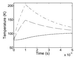
**Fig. 4.** Temperature profiles at the mid point of the: heater (dash-dot line), the insulation between heater and HTS (dashed line), the YBCO-Cu (solid line). The temperature of the insulation between HTS layers is virtually identical to that of the YBCO-Cu layer.
