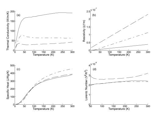
**Fig. 1.** (a), (b), & (c) show measured thermophysical properties; (d) shows calculated Lorentz numbers. Solid lines represent YBCO-Cu, dashed lines YBCO-SS, and dash-dot lines MgB<sub>2</sub>-Ni/Cu/Fe.
