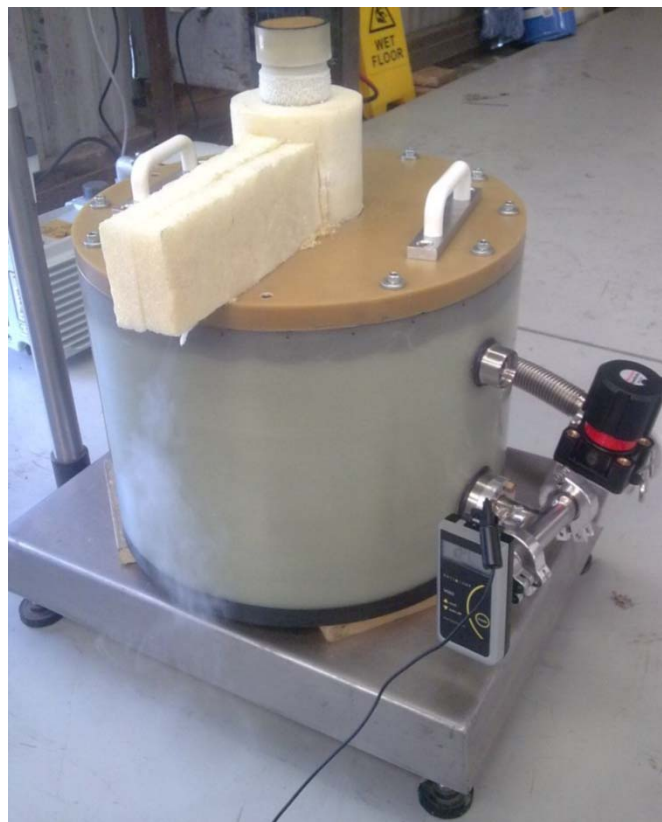
Fig. 2. Small test cryostat on scales undergoing a test. Polyurethane foam encases the fill port and the vent tube to limit heat leak via these openings.
