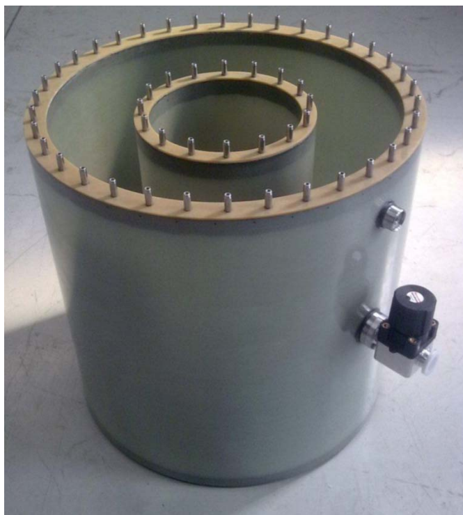
Fig. 1. Composite transformer cryostat for one phase – shown without lid. Note the eccentric central tube.
