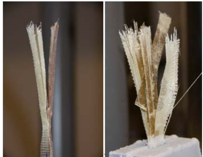
Fig. 4. Fractured tensile specimen of the Arisawa (left) and ACG (right) material.
