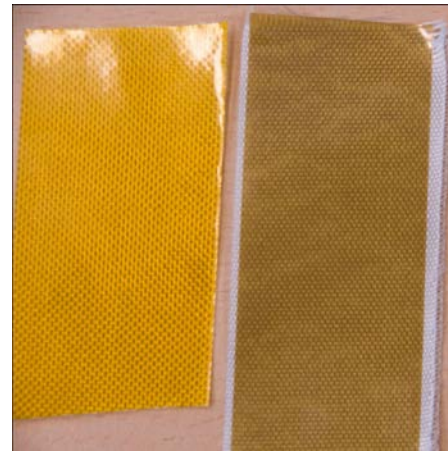
Fig. 2. Bonded glass fiber / polyimide tapes from Arisawa (left) and ACG (right).
