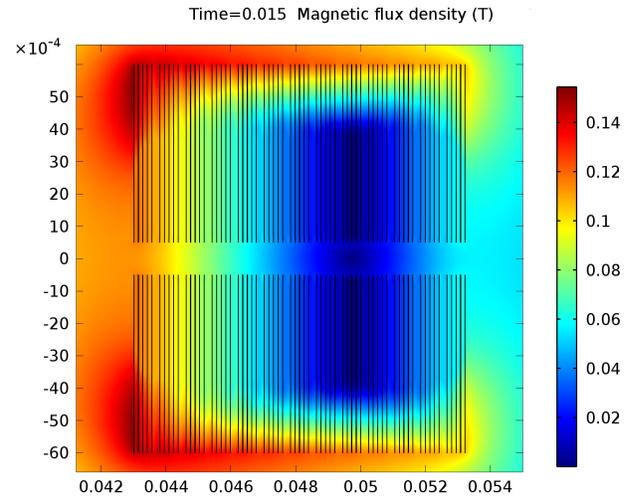
Fig. 3. Magnetic flux density distribution in the coil with turn separation of 0.1 mm. The transport current is 288 A and the distribution refers to the current peak.
