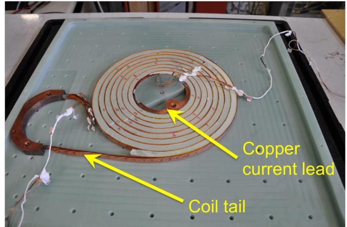
Fig. 7. View of the coil with 10 mm separation between the turns.
