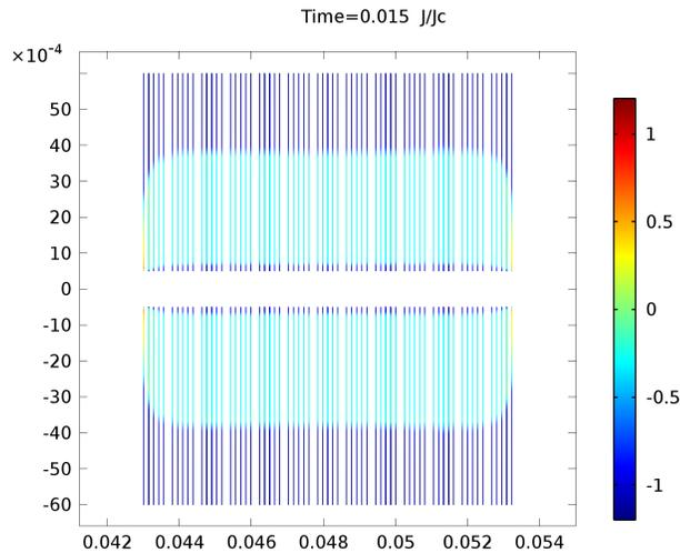
Fig. 5. Current density distribution in the coil with turn separation of 0.1 mm. The transport current is 288 A and the distribution refers to the current peak.
