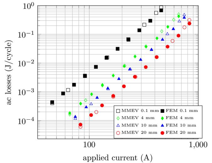
Fig. 2. Computed ac losses as a function of current for the different coil samples.
