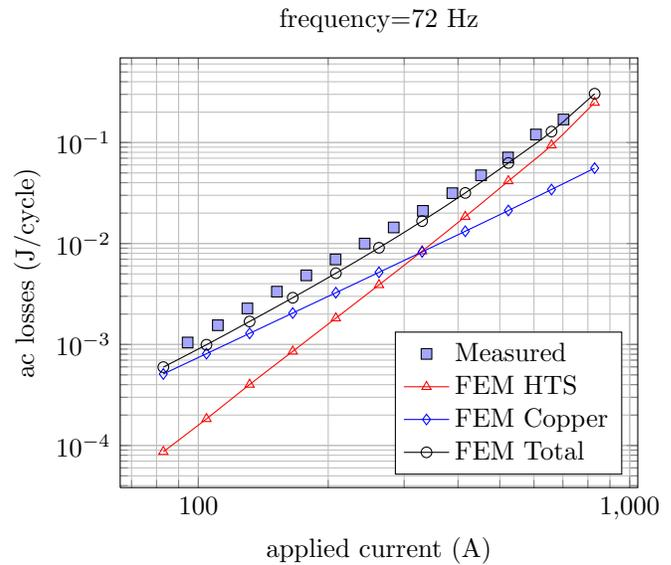
Fig. 9. Comparison of measured and computed ac losses. In the computations, we simulated the presence of a copper turn. The frequency of the current source is 72 Hz.
