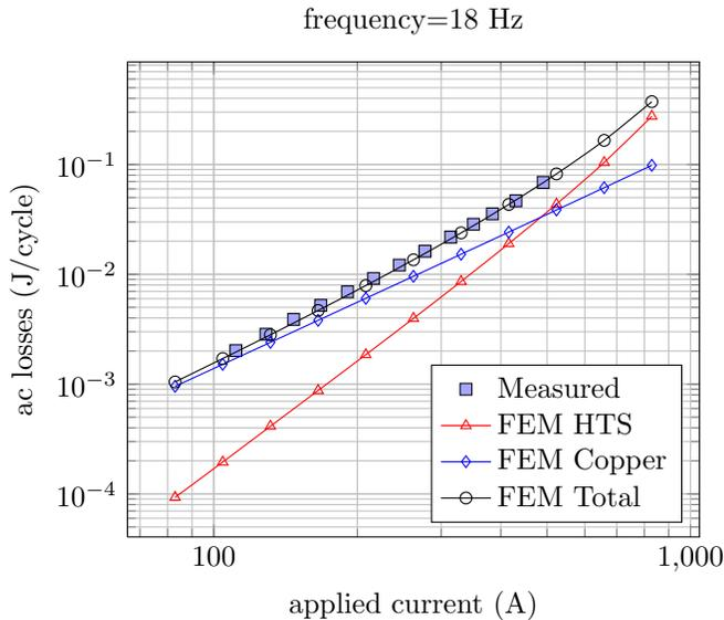
Fig. 8. Comparison of measured and computed ac losses. In the computations, we simulated the presence of a copper turn. The frequency of the current source is 18 Hz.
