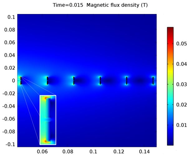
Fig. 4. Magnetic flux density distribution in the coil with turn separation of 20 mm. The transport current is 288 A and the distribution refers to the current peak.
