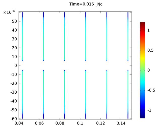
Fig. 6. Current density distribution in the coil with turn separation of 20 mm. The transport current is 288 A and the distribution refers to the current peak.
