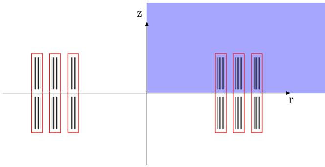
Fig. 1. Schematic view of the cross-section of a coil considered in the simulations (for better readability only three turns are shown). Each red rectangle enclosing ten thin strips represents a turn of the Roebel cable composed of ten strands. For the FEM calculations only one quarter of the full cross-section of the coil (shaded area) is simulated. Not drawn to scale.
