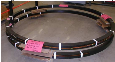
Figure 5. Completed pair of solenoid coils after removal from the winding form and baking.
