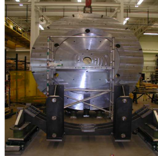
Figure 4. Assembled structure of the return yoke on G-10 posts and the moving-track system.
