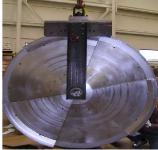
Figure 3. Machined and assembled hill and valley poles attached to a mounting fixture.
