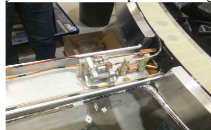
Figure 6. Detail of the shimmed coil in the helium vessel and the diode-resistor assembly.
