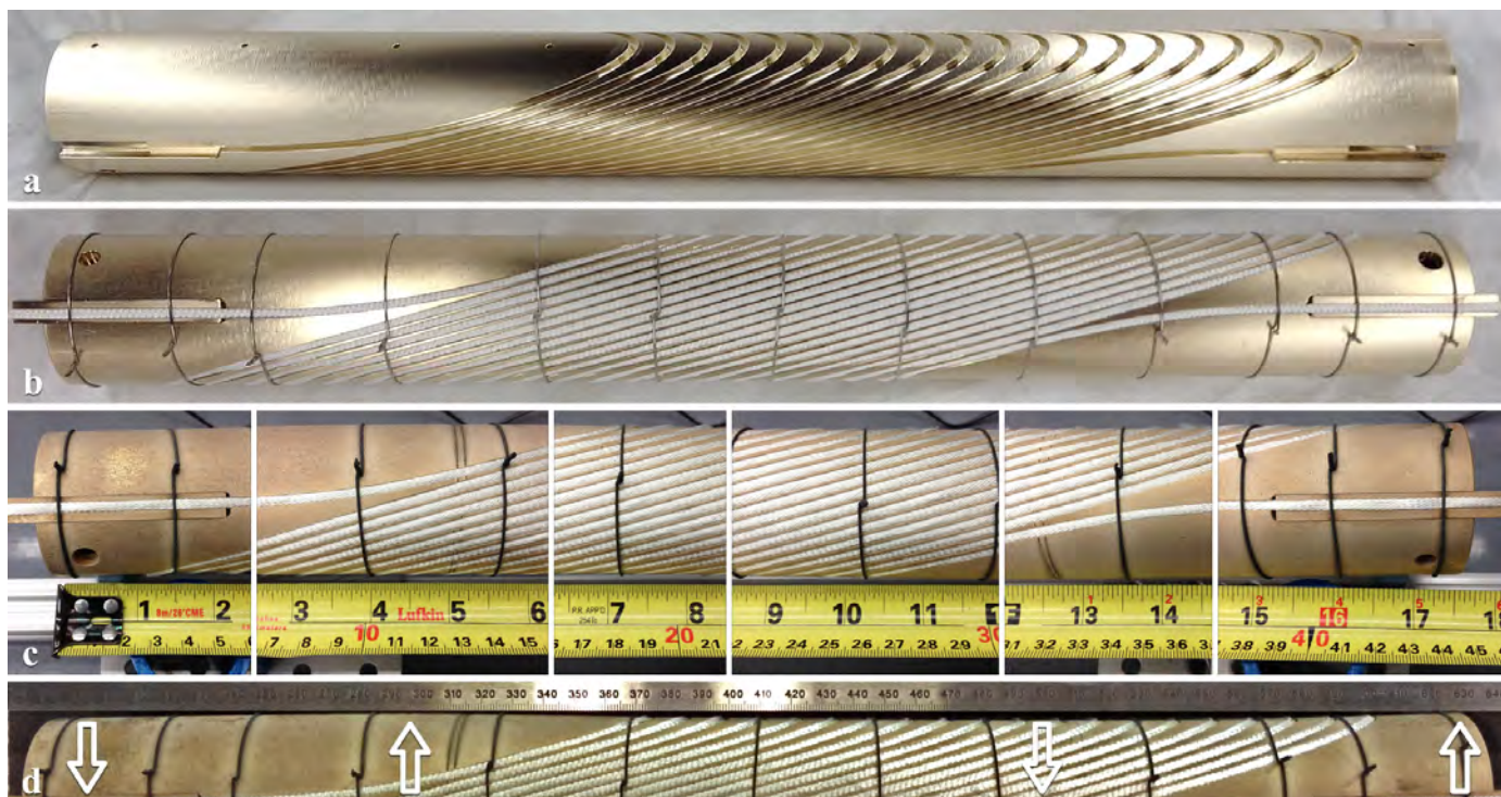
Fig. 4. Inner layer CCT coil for BIN2: a) Machined alloy 642 mandrel with a 2.7 \times 3.0 \text{ mm}^2 round-bottom groove; b) With 6-around-1 alumina-silica sleeve insulated cable made from 0.8 mm Bi-2212 wire, and alloy 954 splice boxes, before reaction; c) After reaction; d) False color picture of the coil after reaction to emphasize the observed mandrel distortion.
