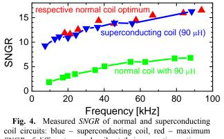
*SNGR* of different normal coils at their respective optimum, green – normal coil with same inductance as superconducting coil.
