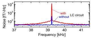
Fig. 2. Measured magnetic field noise density spectra without (blue) and with (red) *LC* circuit. Without the *LC* circuit, the signal and noise were 384 fT and 35 fT/ $\sqrt{Hz}$ , respectively; with the *LC* circuit, the signal and noise were 12.3 pT and 108 fT/ $\sqrt{Hz}$ , respectively.
