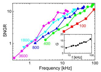
**Fig. 3.** SNGR of *LC* circuits with coils of different windings and different shunt capacitors, measured at their respective resonance. The inset displays the maximum gain *G* obtained with the circuit working best at each frequency.
