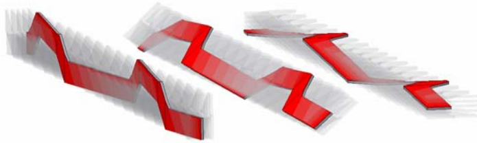
Fig. 1. CAD drawing of a ROEBEL-cable made from 16 strands. One strand is colored to illustrate the full transposition of the strands
