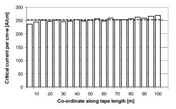
**Fig. 1**. Critical current measured in sections of 100m long YBCO coated conductor. Measurements performed at 77K in self field.
