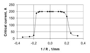
**Fig. 3**. Dependence of critical current in 4-mm-wide coated conductor on 1/R, where *R* denotes bending radius. Measurements performed at 77K and self field. Before bending of the tape (at 1/R=0) critical current amounted to 200.2 A, *i.e.*,  $I_c$  per unit width was 500 A/cm-w. [5]
