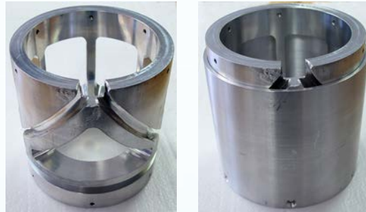
Sample holder for 6 cm diameter cables:
