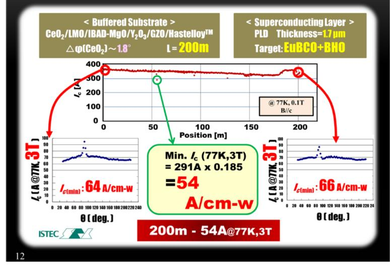
**Annotation**: The new combination of EuBCO+BHO was applied to long tape processing. A reasonably high and uniform performance was confirmed in a 200m long tape.
