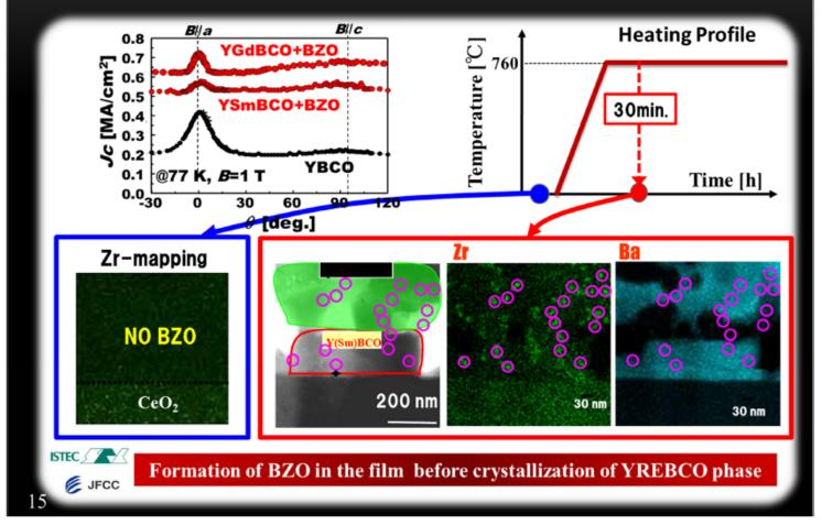
**Annotation**: The introduction of BZO particles was also successfully employed for the MOD process, and the Jc(B) performance could be improved. In order to realize higher Ic(B), the films were quenched during a heat treatment and the microstructure was observed.
