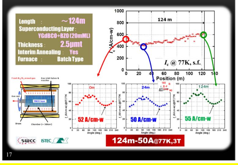
**Annotation**: The new finding was applied to the long tape fabrication of MOD process, and reasonable high in-field Ic values over 50A/cm-width @ 77K & 3T were confirmed in the long tape.
