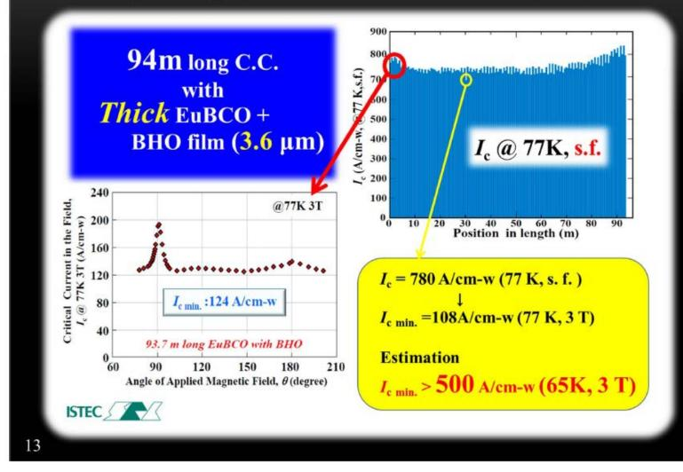
**Annotation**: The thickness of the film in the long tape was enlarged in order to improve the in-field Ic value.
