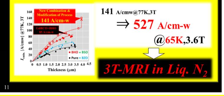
**Annotation**: According to the progress in the EuBCO+BHO, it can be expected that the 3T-MRI can be operated in Liq. N2 by utilizing this performance.
