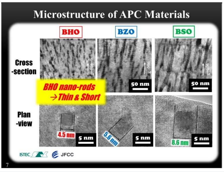
**Annotation**: The observation of the microstructure tells us one reason for the higher Ic(B) performance: The diameter of the BHO rods is smallest and shortest.
