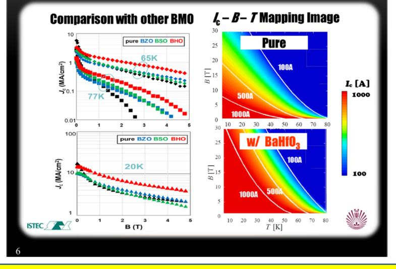
**Annotation**: The BHO addition has several desirable features. One of them represent the advantageous Ic(B) properties for a wide range of temperatures and magnetic fields.
