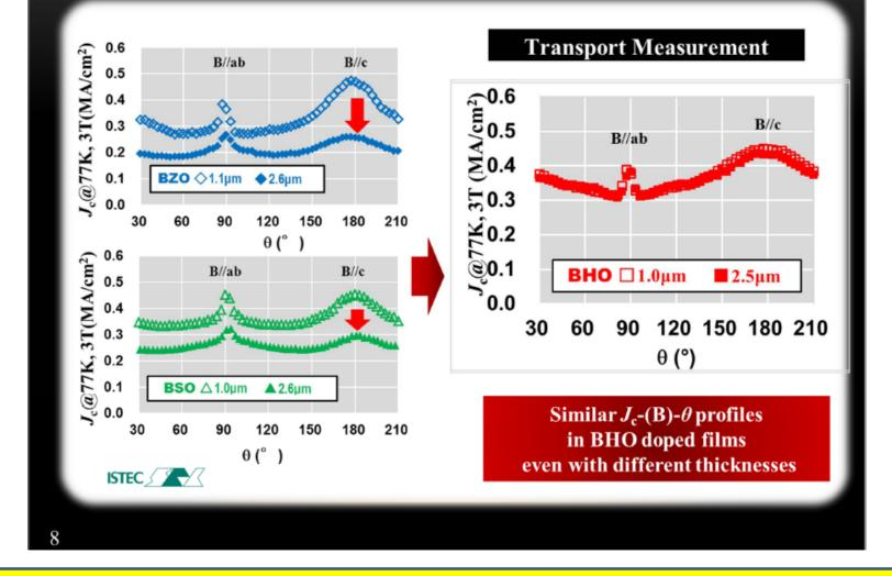
**Annotation**: Another desirable feature is the performance in thick films. There is no difference between the Ic-B-theta properties of thin and thick films for the BHO addition.
