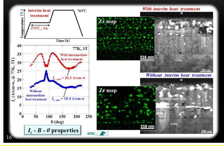
**Annotation**: Through the investigation of the influence of the heating pattern on the in-field performance, it was found that the addition of the interim annealing step is effective to improve the Ic(B) performance through the finer and well-dispersed BZO particles.
