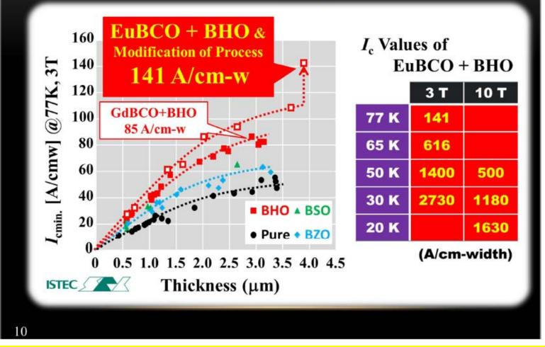
**Annotation**: Most recently, we found that a new combination of EuBCO and BHO is even more effective to suppress the degradation of the in-field Jc with increasing thickness. The Ic value of 141A/cm-width @ 77K and 3T, which is the highest value in the world, was obtained.
