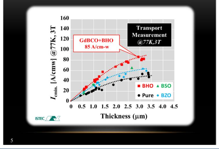
**Annotation**: Clear improvement in the Ic(B) performance due to the additions of BZO & BSO can be confirmed. However, the Ic(B) values become saturated with increasing thickness.
