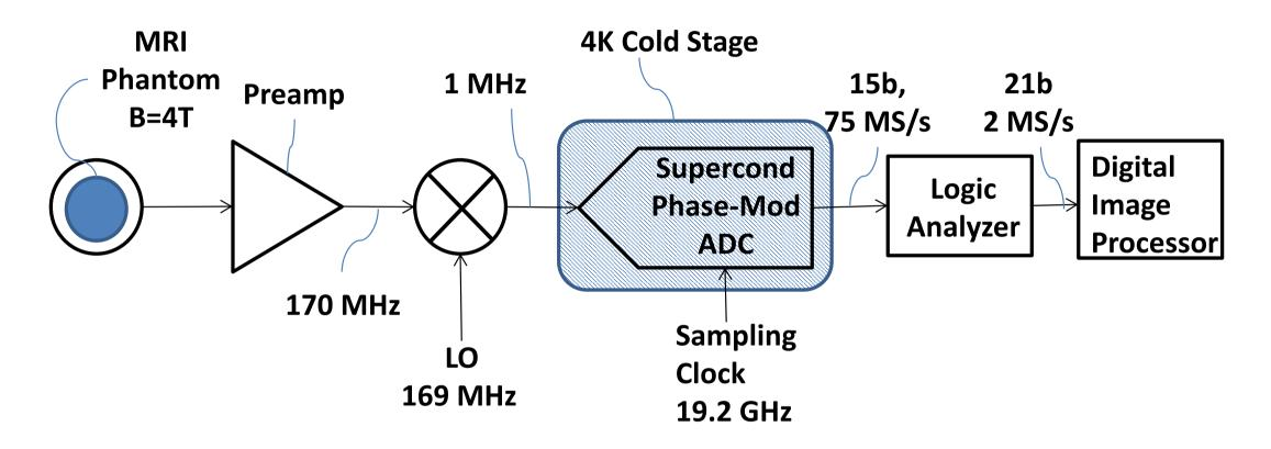
ADC substituted for the 16-bit ADC of a Bruker Avance 4T small-animal MRI system at Yale Magnetic Resonance Research Center.
