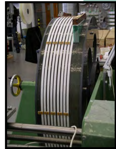
Roebel cable ready for testing at Siemens Corporate Technology
