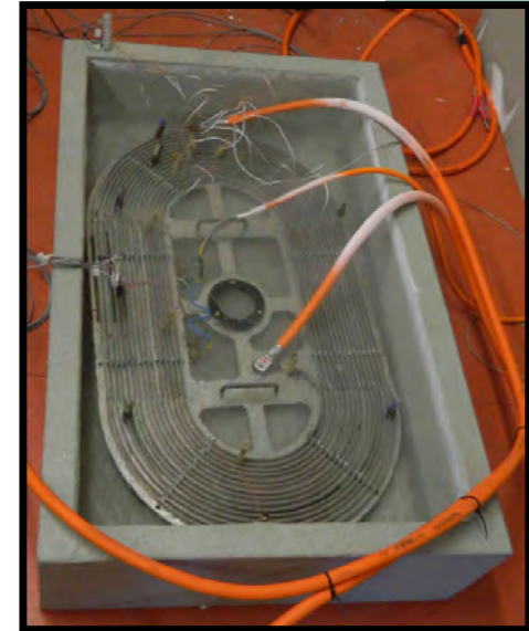
Spiral racetrack former for testing strands up to 30 m
