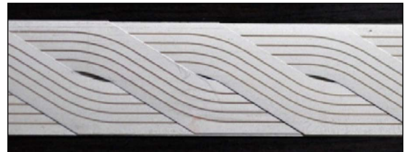
Roebel Assembled Coated Conductor Cable with filaments
