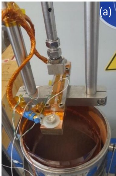
(a) Sample holder for I_c vs transverse stress measurements with (b) 1 mm-wide and (c) 5 mm-wide pressing tool.
