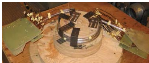
HTS Conductor bending
