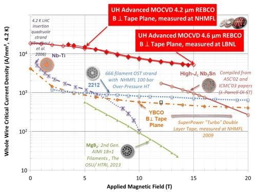
$J_e$  of 4+ µm REBCO 5X Nb<sub>3</sub>Sn @ 14 T
